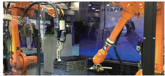
图3 多机器人增材减材混合设备 Fig.3 Multi-robotic machine performing additive and subtractive machining simultaneously
